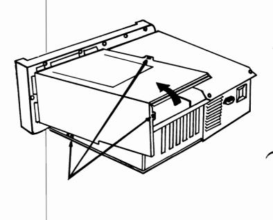
$\mid$   $\blacksquare$  Slide the cover forward back onto the chassis.
