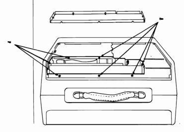
■ Put the metal plate back into place and replace the seven screws.
