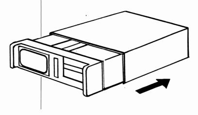
■ Remove the screws from the metal shield on the right hand side of the computer. Remove the shield. You will find the expansion slots under this shield.
