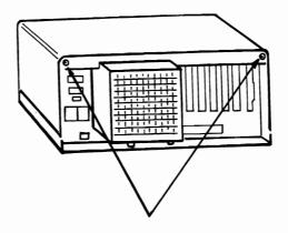
■Slide the cover forward to release it from the chassis, then lift it off.
