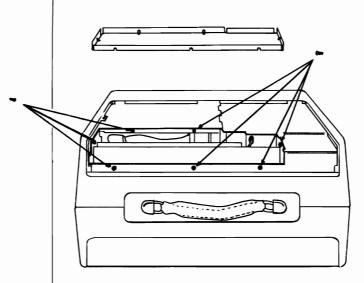
■Insert the tabs on the back of the cover into the slots on the top of the chassis. Gently push down until the cover snaps shut.
