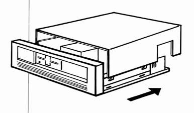
■Lift the cover back onto the computer chassis.
