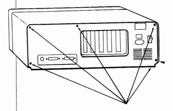
■Slide the cover forward slightly, then lift straight up slowly. Connecting cables for the disk drive are attached directly to the cover and should not be removed.
