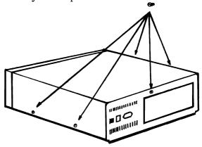
■ Slide the cover forward, then lift it up and remove it.
