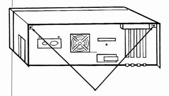
■ Slide the cover toward the back slightly until the cover is released from the chassis, then lift it off.
